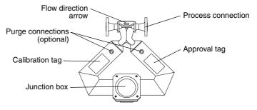
Flow direction arrow Junction box Calibration tag Flow direction arrow Calibration tag Flow direction arrow Purge connections (optional) Approval tag
